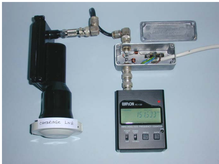
Figure 4 – 10GHz frequency measurement
